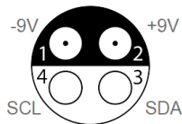
Probe’s power supply pin assignment “cable view”
